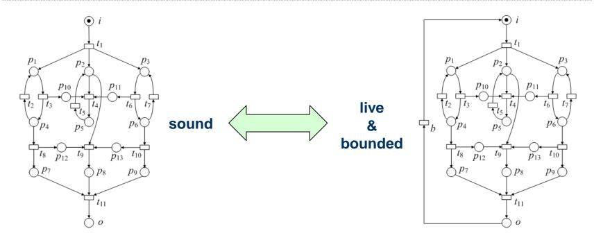
**Corollary**: Let N = (P, T, F) be a WF-net, and  $(N^E, M_0) = (P, T \cup \{b\}, F \cup \{(b, i), (o, b)\}, i)$  be bounded. Then, N is sound if and only if  $(N^E, M_0)$  is live.
