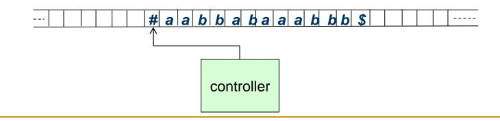
**Step1**: use places to represent the tape information, machine state, and read/write head position.
